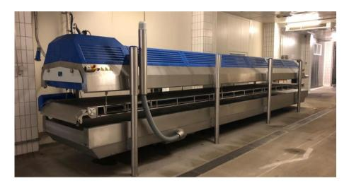
Linde Cryogenic tunnel freezer, with touch screen control, retention time: 1.5 min - 50 min, suitable for a full range of fresh & cooked food products.
