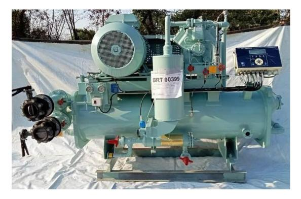
Never installed reefer set. Based on Bock FX16 Compressor. Complete with controller. The E-motor is ABB Marine 63kW 400V/3 phase / 60Hz.
