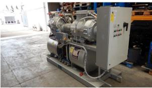
Very well maintained Chiller PAC based on a SMC 106E. On this unit is a e-motor of 132 kw installed and a complete controller unit. The refrigeration side is controlled by a UNISAB II.
