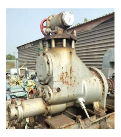
A original Booster version of the MK1 Sab 163. The BS is has an longer body and no balance pistons . For users of a MK1 A63 BS a great opportunity to get a spare compressor , which fits on their SAB 163 MK1 BS unit. This model is long time out of production.
