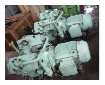
Capacity 200 m3/h Pressure: 25 bar 1770 RPM (max) Common base frame
