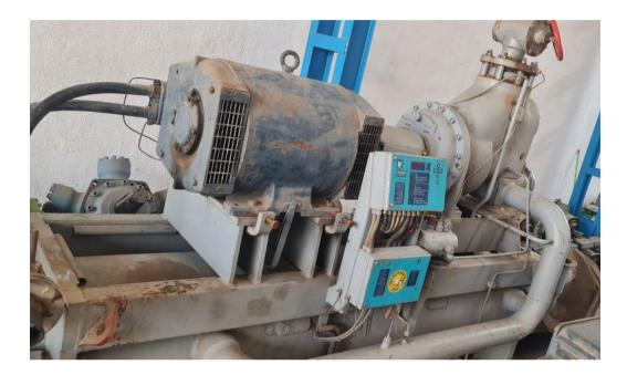
Available SAB 163 mk1 BM, the booster version of the SAB 163 mk1 The compressor is running removed of the unit.
