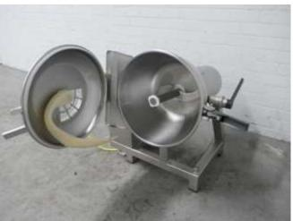
Suitable for Meat, process meals, salads, dressings and more. Bowl capacity: 45 lite- 3 speed rotation: 700, 1450 and 2900 RPM. Complete overhauled –weight: 230 kg- dimensions: 750 x 550 x 1150 mm
