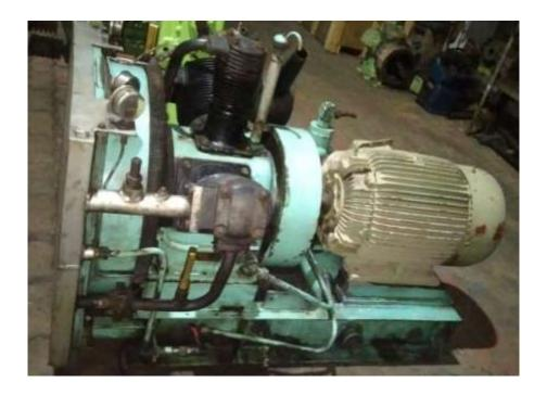
Capacity 118 m3/h Pressure: 30 bar 1750 RPM (max) Common base frame
