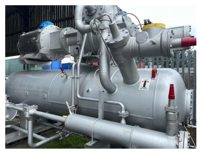
Brand new overstock Compressor unit based on a Sabroe 283E compressor . Due to change of plans never installed. E-motor 315 kW . Unisab pro III controller – year of build 2017. Complete unit.
