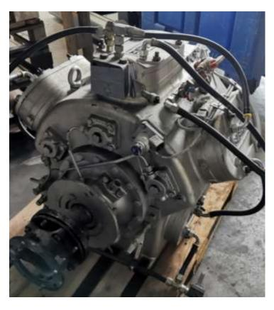
Available: 2 Bare shaft compressor block SMC106E. year of construction 2007. The units are suitable for NH3.
