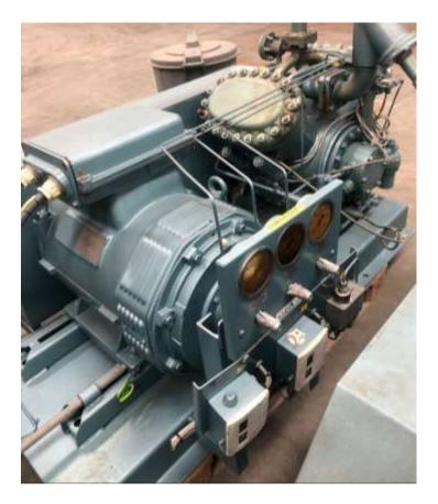
**Available:** 1 Grasso RC 49 in very good condition. E-motor 55 kw , direct driven. Complete unit – year of construction 1999 . The units were running on NH3.
