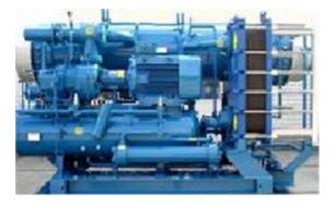
This filter house you find on many compressor units with Howden XRV compressors and low stage WRV units.
