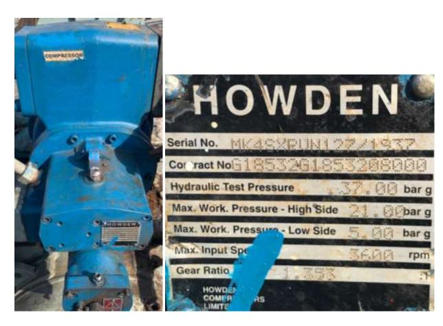
A bare shaft Howden Mk4S/XRV127 R3 of Nodular iron. If you require a spare compressor this is a perfect time. The compressor can be delivered as it is or overhauled.
