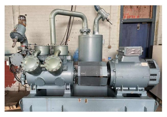
Very maintained Grasso RC612E compressor unit – direct drive of 2002. The unit is suited with a 200 kW E-motor. The RPM are 1480. The models of Grasso RC 612E are design for 1500 RPM. A stabel investment is compressor unit, which proven themselves more than 40 years. The max swep volume is 1195 m3/h
