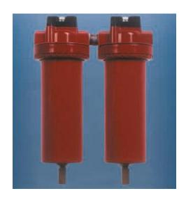
De eliminizer combo produces clean , dry and oil free air at the supply point. The first phase is water reduction by the eliminizer. The second phase is the oil reduction by an effective coalescing element. Effectivity till 0,01 micron The recommended point of installation is max. 5 meters from the air supply point.
