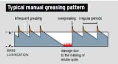
By manual Lubrication the process starts always with over lubrication on the lubrication points.
