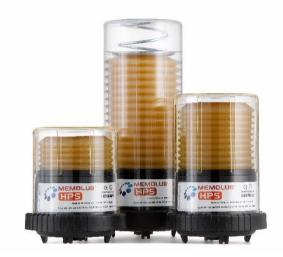
The Memolub HPS can be installed direct on 1 lubrication point or on distance with flexible lines till a distance of maximal 8 meters. With one lubricator can 2 till 8 lubrication points be serves by the use of splitter (2 points) or Distributor blocks of the DB- range. (4-6-8 points)
