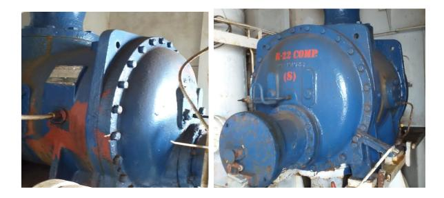
A very nice strong Howden WRV255/130.58 was original running on R22. By overhaul ready to be modified in a NH3 or Freon compressor . Even with a coldores double shaft seal suitable for Propane and propylene. Ideal spare compressor .
