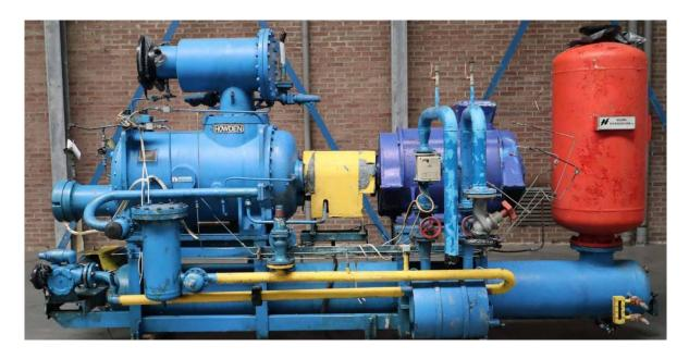
For me a well-known oldie – the compressor is a the very strong MK4/WRV255/220.26 –a real booster compressor with a working length of the rotor of  $2.2 \times 25.5$  cm.
