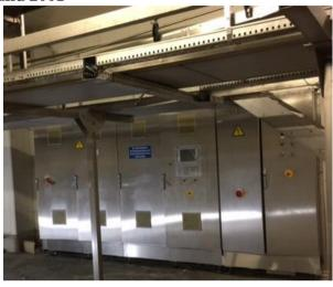
Well maintained Heinen MES 12/22-5800S multilevel Carton box Freezer - year of build 2001. -Stainless steel floor, Siemens touch screen Control, ideal for Freezing packed goods, Tiers:14 Levels / 22 Shelfs, Product gap: 435 mm, Belt width 5800 mm, Capacity: 5000 kg/h (57 kcal/kg), Refrigerant:NH3, Cooling power: 500 kW, Evaporator 3 pcs type: Goedhart PLK.S 1285 M2, Power: 3 x 400 V / 50 Hz / 160 kW, Dimensions: 24510 mm x 9610 mm x 7900 mm, Weight 42000 Kg
