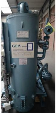
The oil separator is GEA version with oil separator elements in last stage. The oil separator is suited with a standby heater.
