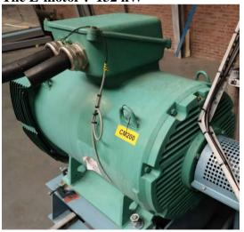
The E-motor is a Leroy Somer PLS 315L-T. construction: B3- IP 23. The capacity is 250 kW at 2970 RPM The year of build is 2002.
