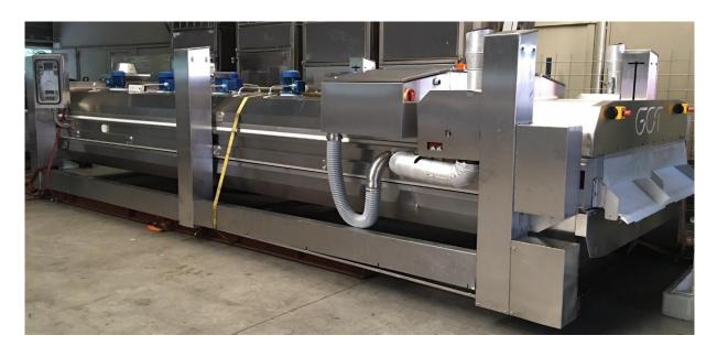
A nitrogen tunnel freezer in good condition, double belt – speed is spate controllable, Product gap: max. 150 mm, Belt width: 2 x 700 mm, Belt length 6600 mm, Refrigerant: Nitrogen, Power 3 x 400V / 50Hz / 16kW, Dimensions7610 mm x 2300 mm x 1800 mm. Weight:3450 Kg.
