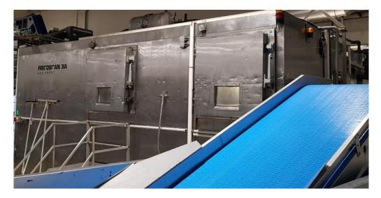
The Frigoscandia Flo freeze MX 52 freezer with Ai Defroster system (ADF), new switchbox and controller fitted by JBT in 2018.
