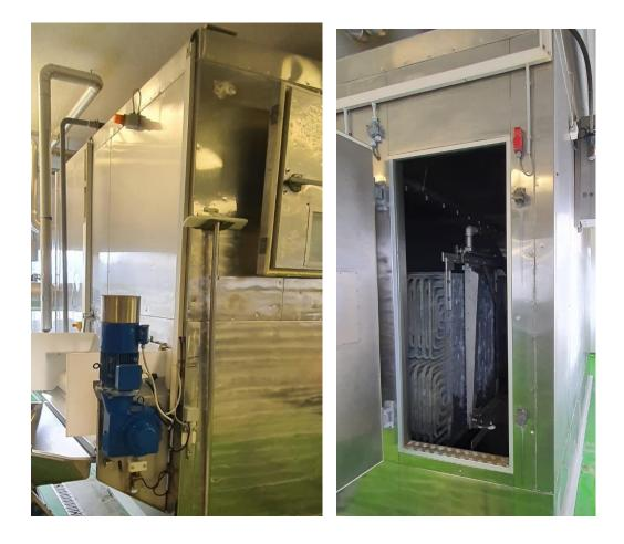
The Frigoscandia Flo freeze MX 32 freezer will be available in May 2021. This Freezer will be offered complete refurbished without isolation panels. New Isolation panels are available optional . The Capacity is nominal for peas 1950 Kg / hour
