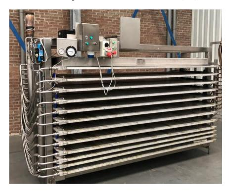
Horizontal plate freezer model of Freezertech Services of 2015 – 11 stations – dimensions 2450 x 1120 mm- design temperature  $-40^{\circ}\text{C}/ + 40^{\circ}\text{C}$ - test pressure 29 bar – design pressure 22 bar
