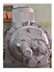
The SAB163 Mk1 auto Vi can be delivered as Male driven (HM) of be modified as Female driven (HF)
