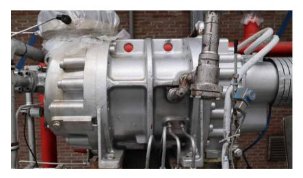
The compressor block VMY346NR has a Sept volume of 2708m3/hr /50HZ Own main full flow oil pump. Eco
