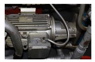
The unit is suited with 2 oil pumps – the external is used by start to build –up the oil pressure and prepare for lubrication to start.
