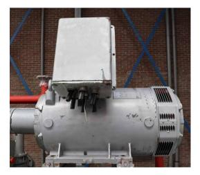
The E-motor is a well-known model . On 400V at 2950 RPM (50 Hz) the duty is 450 kW. Even on 460V at 3565 RPM (60 Hz) the duty is 520 kW .
