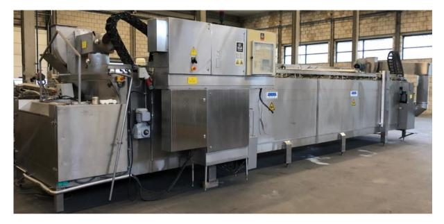
Interesting Product Liquid Co2 tunnel freezer, 3 belt system at different heights, product gap: 120 mm, Belt width gross 1220 mm/ nett 1200 mm. Infeed height 1400 mm, out feed height: 525 mm, Refrigerant : liquid CO2, Power3x 800 V / 14 kW, Dimensions 10500 mm x 2650 mm x 2600 mm (closed) / 10500 mm x 2650 mm x 3540 mm (opened), Weight 6000 kg
