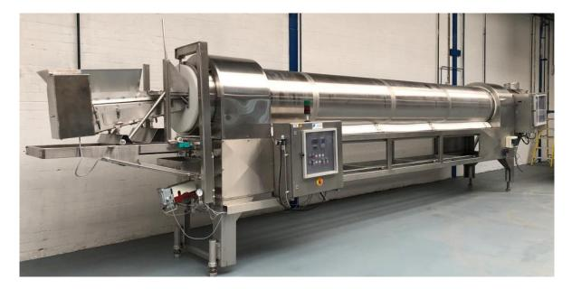
**Interesting special product CO2 tumbling freezer od the well-known builder Dutch CES.** Nice solution for chilling / freezing of Small bulk products during a tumbling process. Food products like vegetables, fruits, chopped meat , fish and poultry . Or a total other process industrial products in cooling processes / freezing for the next step in production .
